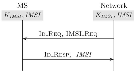
Fig. 2 Identification procedure. The identity of the mobile phone is sent in clear on the radio path
