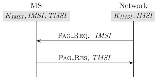
Fig. 4 IMSI paging procedure in UMTS: the paging request message is sent on a common radio channel and contains the identity of the paged mobile station (in this case the IMSI) in cleartext. The paging response message contains the mobile phone’s temporary identity TMSI and is sent in clear on a dedicated channel
