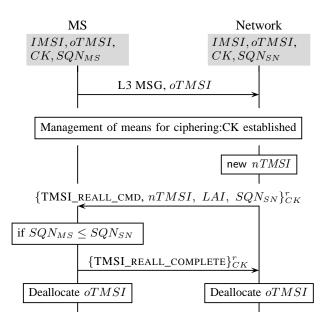
Fig. 8. TMSI Reallocation Procedure SQN Fix
