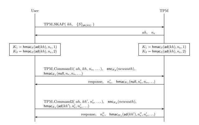
Fig. 2. Establishing a session using Session Key Authorisation Protocol, and executing two commands in the session. The session is established relative to a loaded key with handle kh. Command1 uses that key, and therefore does not need to cite authdata. Command2 uses a different key, and cites authdata in the body of the authorisation HMAC.
