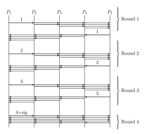
Fig. 1. Messages in our Main protocol when n=5. In order to reduce clutter, each line in the figure represents a set of messages broadcast by a single signer to a set of signers. For example, the first line stands for 1-level promises sent by  $P_1$  to all other signers.
